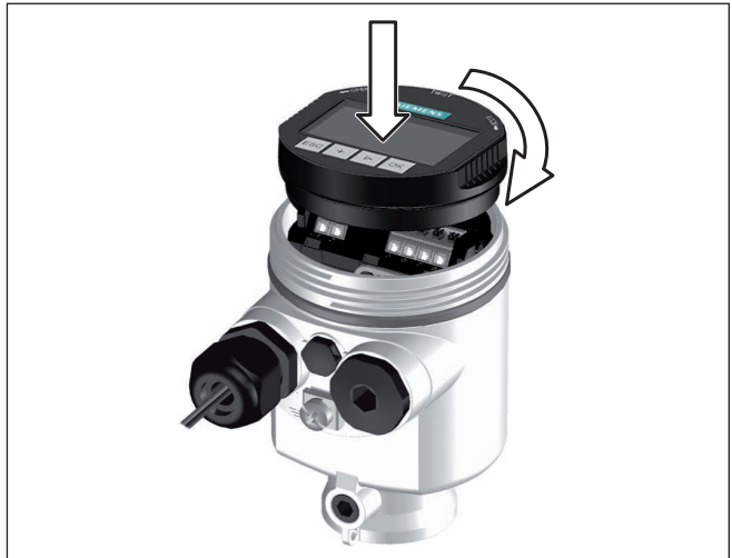
Fig. 15: Insertion of the display and adjustment module with single chamber housing into the electronics compartment
